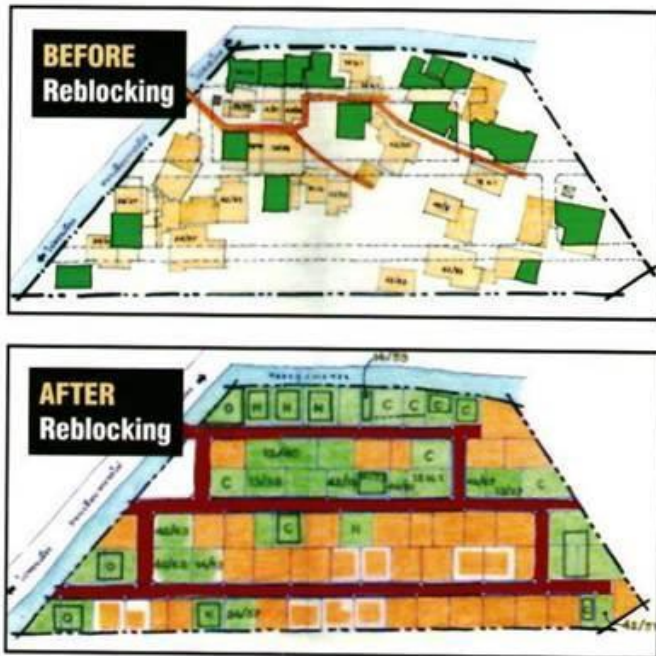
Reblocking at Charoenchai Nimitmai in Bangkok, with straightened and widened lanes and rebuilding of many of the houses.
